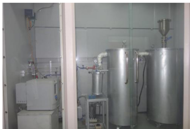
Fig. 2. Smelting and purification equipment for preparation of molten FLiNaK salt.
